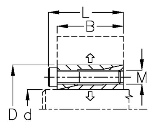
$\begin{array}{lll} \text{B mm} & = 21 \\ \text{d mm} & = 17.00 \\ \text{D mm} & = 35 \\ \text{Fit tolerance} & = \text{Aksel h8, Nav H8} \\ \text{F kN torque} & = 8.0 \\ \text{L mm} & = 25.0 \\ \text{M mm} & = M4 \\ \text{P N/mm2 surface pressure on shaft/hub} = 60 \end{array}$
